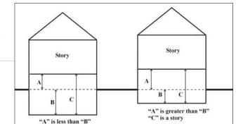
the Foundation and the surface of the next floor, or if There is no floor above, then the ceiling next above.
